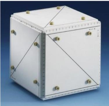
Auxiliary Inserts for ionization chambers for Farmer and Compact chamber types
